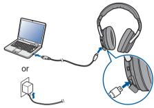
The Charge/NC indicator blinks during charging. It takes approximately 3 hours to charge the headphones. (The duration time differs depending on the charging output.)
