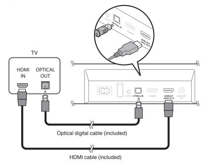
• Line up the optical digital cable with the shape of the terminal to insert.
