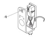
(3) Tighten the screws with a screwdriver to secure the cartridge to the head shell.
