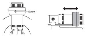
If your cartridge and head shell are too heavy to keep the tone arm parallel to the record with the counterweight alone, attach the included subweight to the tone arm. (127 p. 15)
