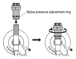
· Mount the counterweight so that its stylus pressure adjustment ring is facing the front.
