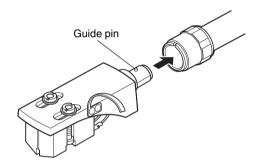
2 Turn the lock nut in the direction of the arrow to secure the head shell.
