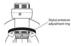
8 Turn the counterweight in the direction of the arrow to set the right cartridge stylus pressure.
