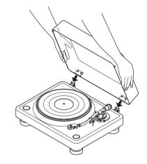
• To remove the dust cover, open the dust cover all the way and then pull it in the opposite direction to that indicated by the arrows.
