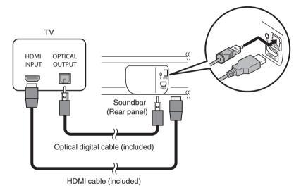
• Line up the optical digital cable with the shape of the terminal to insert.
