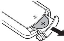
3. Remove the old battery, then insert a new coin-shaped lithium battery (CR2025) into the battery compartment so that the + symbol engraved on the battery faces upwards.
