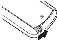
2. While pushing the catch lightly to the right, pull out the battery case.
