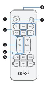
Power button (𝔅) Turns the sound bar power on/off (standby). (𝔅 p. 23)
